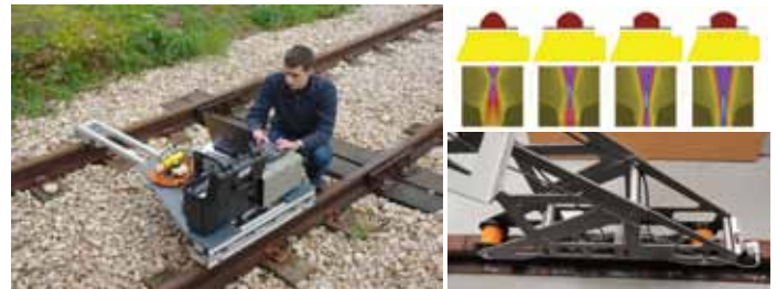
ACFM and PA walking stick for quantification of surface breaking defects and signal output screenshot indicating the defects detected and quantified.
